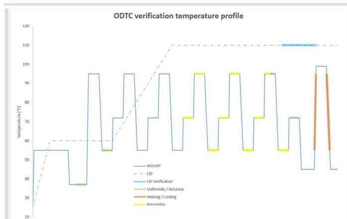
**Fig.29: Temperature profile during verification**
