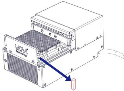
**Fig.24: Block removal**
