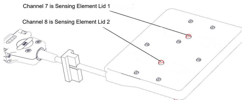
**Fig.41: OVT Channel corresponding sensing elements for ODTC® Lid**
