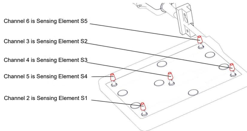
**Fig.40: OVT Channel corresponding sensing elements for ODTC® Mount (VCM)**
