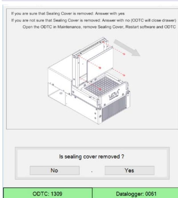
Fig.23: Confirm whether the Sealing Cover is removed
