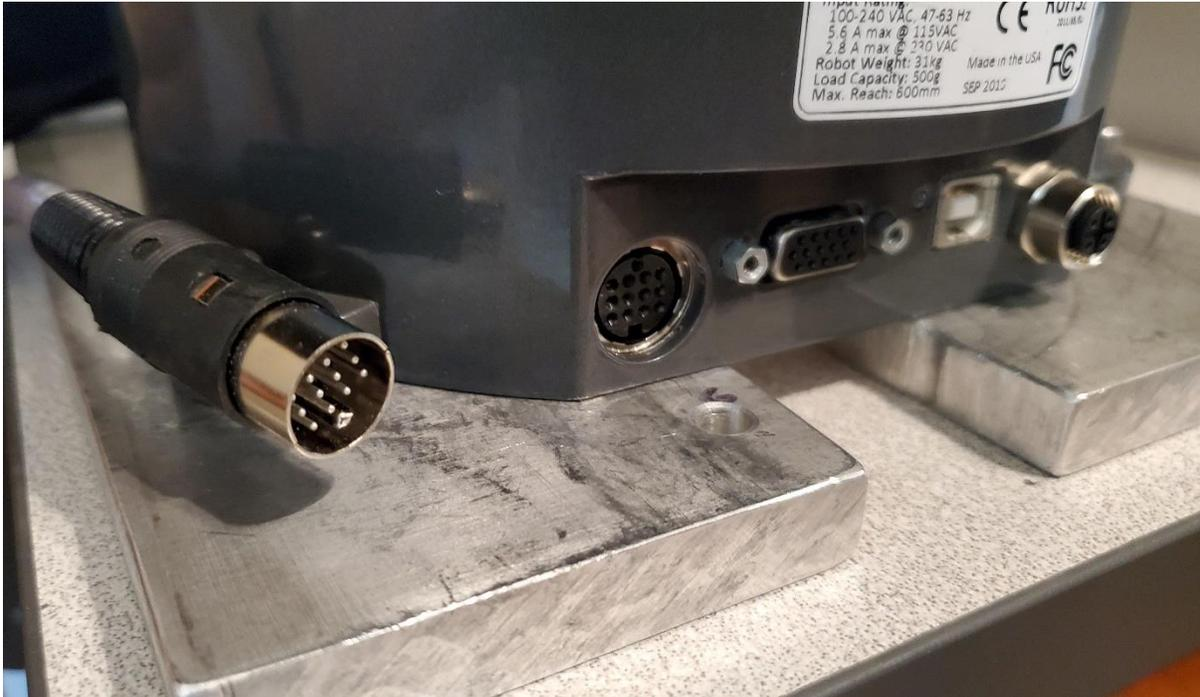
Updated Power Supply Connector for KX-2 Rail & Newer Robots:
