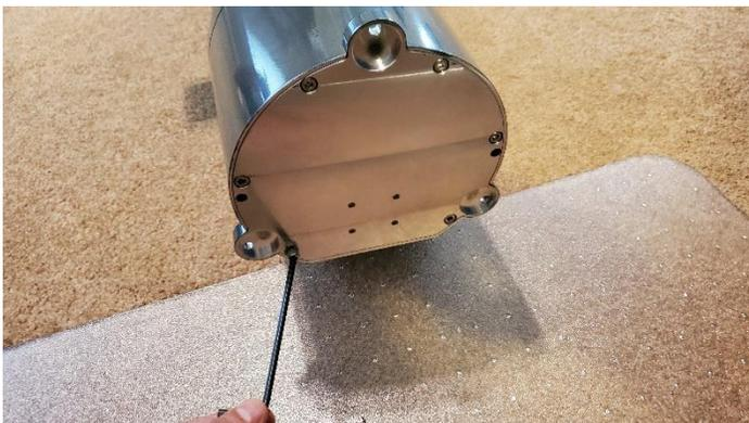
Note: Before proceeding, verify all four M2 screws are removed. If any of these screws are left installed, damage to the shoulder motor drive may occur during the next step. If the M2 screws are left installed and the shoulder motor drive detaches from the PCB in the following step, then remove the drive from the bottom plate and reinstall it on the PCB. Be sure to line the motor drive pins up with their corresponding connectors and confirm none of the pins are bent.
